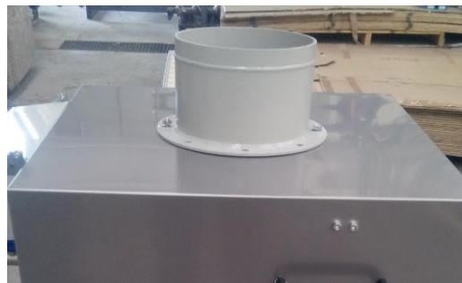
Fan Connection Flange is mounted with bolts on the fan intake hole of top cover and assemble the fan connection flange to the filter cover with seal.
